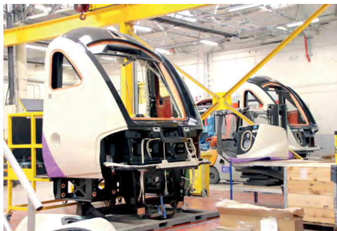
Cabs for the Class 345 under construction in the Bombardier cab shop at Derby.
