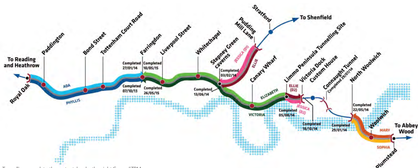
Tunnelling complete: the routes taken by the eight Crossrail TBMs.
