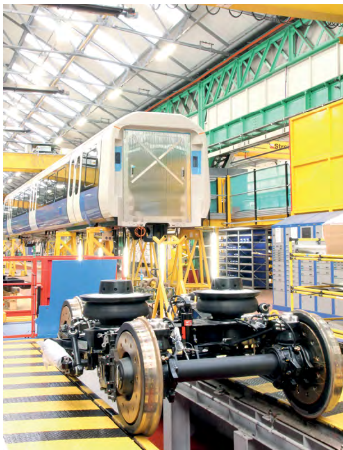
Class 345 bodyshell on the Derby production line, with a FLEXX Eco Bogie in the foreground. Production photographs courtesy of Bombardier
